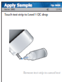
7 Touch drop from QC bottle to strip. Result will appear within 6 seconds.
