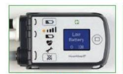
Yellow or Red Battery Alarm: Need to Change Batteries. See changing batteries section on next page.
