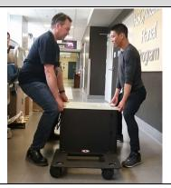
Lock the brakes on the cabinet. ET and Assistant squat or half kneel on either side of the control unit. On a specified count, ET and Assistant lift and shift body weight to slide the control unit into the cabinet with back straight and arms close to body.
