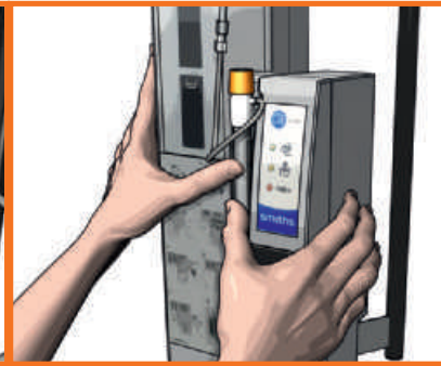
8 Press Gas Vent/Filter Assembly into #4 block.
