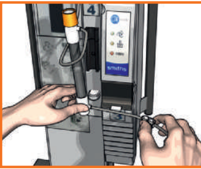
4 Move the pinch clamp connector on the Patient Line of the Gas Vent/Filter Assembly next to the Luer connector. Close the pinch clamp.
