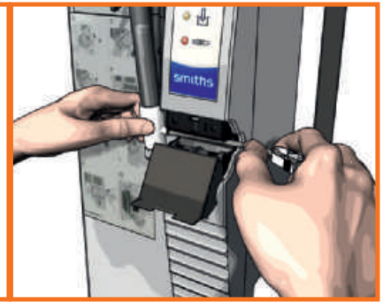
6 Insert the Patient Line in the Clamp Slot and push it back into the slot.
