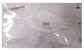
Label the pouch with the decontamination cycle count, and seal it.
