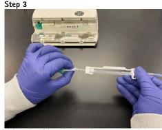
Using the IPA pad, wipe the segment of the pump tubing between the silicone pump segment and the green, set-based anti-freeflow protection clamp
