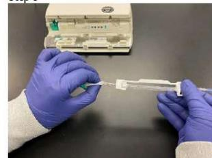
Using the IPA pad, wipe the segment of the pump tubing between the silicone pump segment and the green, set-based anti-freeflow protection clamp
