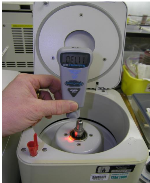
Defeated lid lock mechanism.
