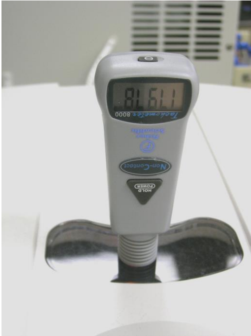
Reading Cytospin through window in lid.
