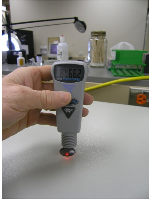
Reading Cytospin through window in lid.
