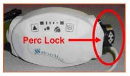
**Driveline Connection:** The Perc Lock must be "unlocked" in order for the driveline to be removed in a controller exchange. The Perc lock remains in locked position once the driveline has been fully inserted.
